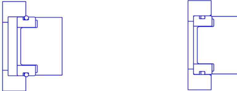
INSTALLING MAGNET INTO HOUSING USING DRIFT
